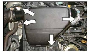
4. Remove the three bolts that secure the intake plenum to the engine and loosen the throttle body hose clamp.
