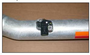
17. Install the mass air sensor into the K&N® intake tube and secure with the provided M4 button head allen bolts as shown.
