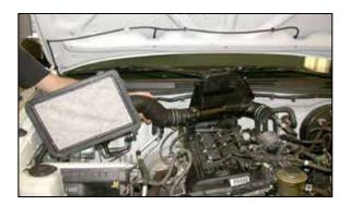
5. Unlatch the upper air box retaining clips, disconnect the fuel pressure regulator and crank case vent hoses and then lift the intake tract off of the throttle body as shown.
