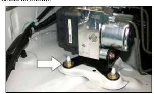
11. Remove the ABS pump mounting nut shown. **NOTE: This nut will be reused.**
