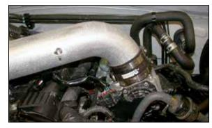
18. Install the K&N® intake tube onto the throttle body and align with the tube mounting bracket that was installed in step #14.
