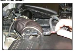
2. Disconnect the mass air sensor electrical connection and unclip the three wire harness retaining clips from the intake plenum.
