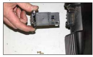
16. Remove the two mass air sensor retaining screws and then remove the mass air sensor from the factory air box.
