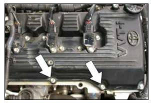
13. Remove the two valve cover bolts shown. **NOTE: These bolts will be reused.**
