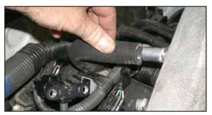
Install the provided crank case vent hose onto the valve cover port and then onto the K&N® intake tube and secure with the provided hose clamps.
