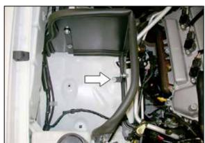
12. Install the heat shield onto the vehicle and secure with the provided hardware and the nut removed in step #11.
