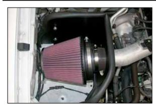
25. Install the air filter assembly onto the intake tube as shown.
